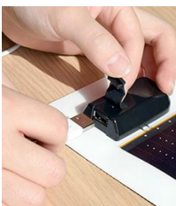
(1) Charging from Solar sheet to LED lantern
